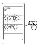
Component names are displayed. The labels for which a series of commands is programmed stay lit and others flash.
